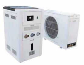
The indoor unit is consist of water pump, water reservoir and evaporator while the outdoor unit consist of compressor. fan and condenser, which can discharge all heat and noise outside. Split type design improve comfort and reduce the noise, at the same time enhance the cooling capacity. Their large refrigeration capacity with steady operation also used as a central supply of cooling water for labs or complete buildings.
