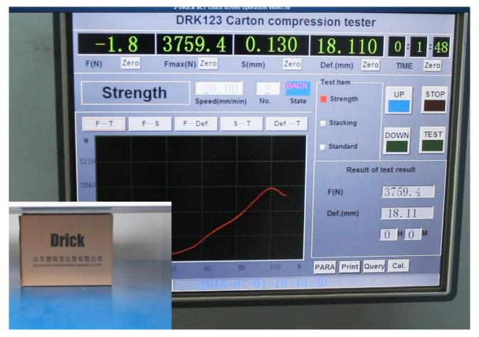
Curve and graph showing the changing of the compression strength force during the test period
