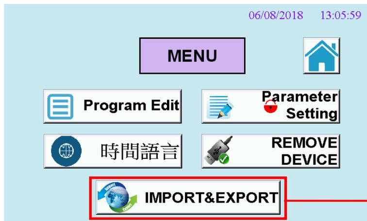
Plug in a USB device to HMI, click **IMPORT&EXPORT** button with password
