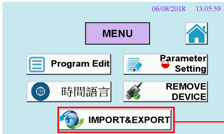
Plug in a USB device to HMI, click **IMPORT&EXPORT** button with password inputting
