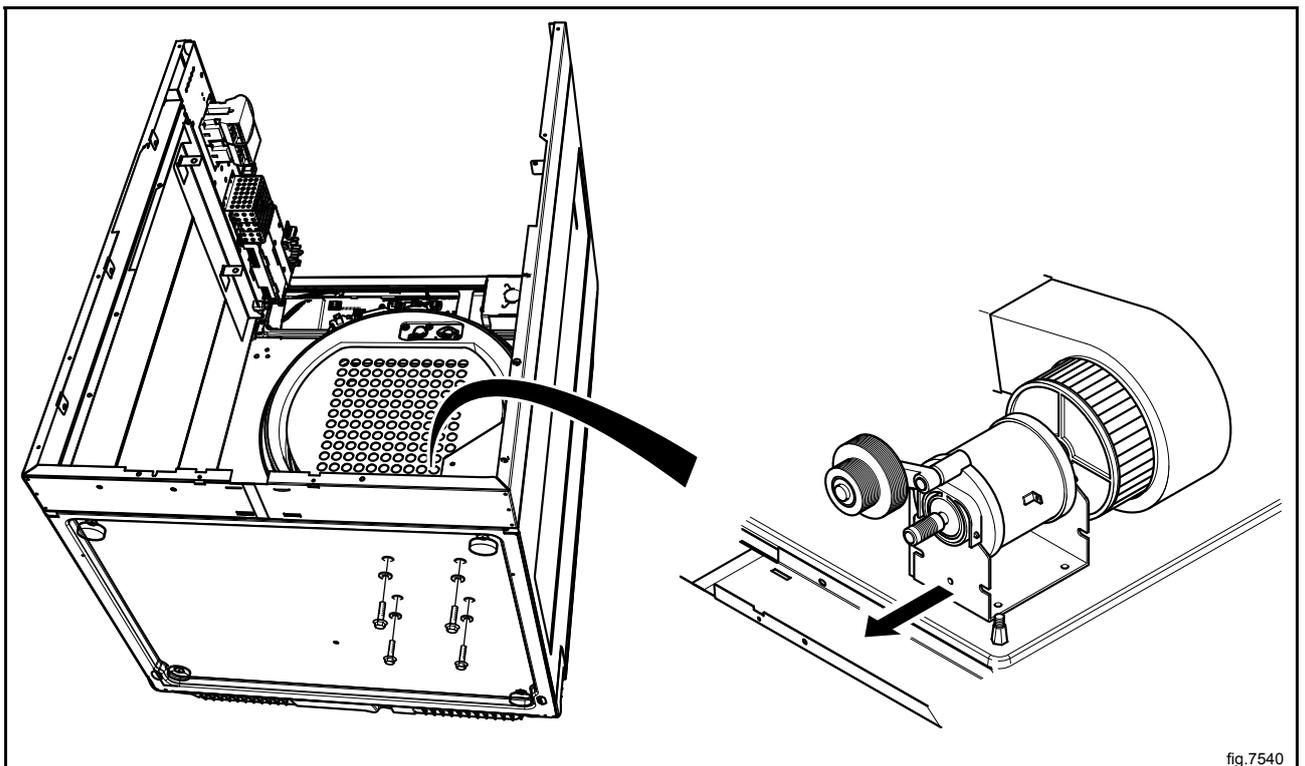
Demount the fan from the motor by loosening the set screw. The set screw can be accessed through a hole in one of the blades.
