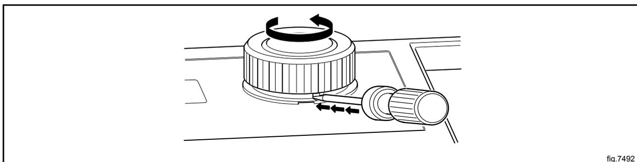
Continue turning a quarter of a turn until it is possible to remove the control knob.
