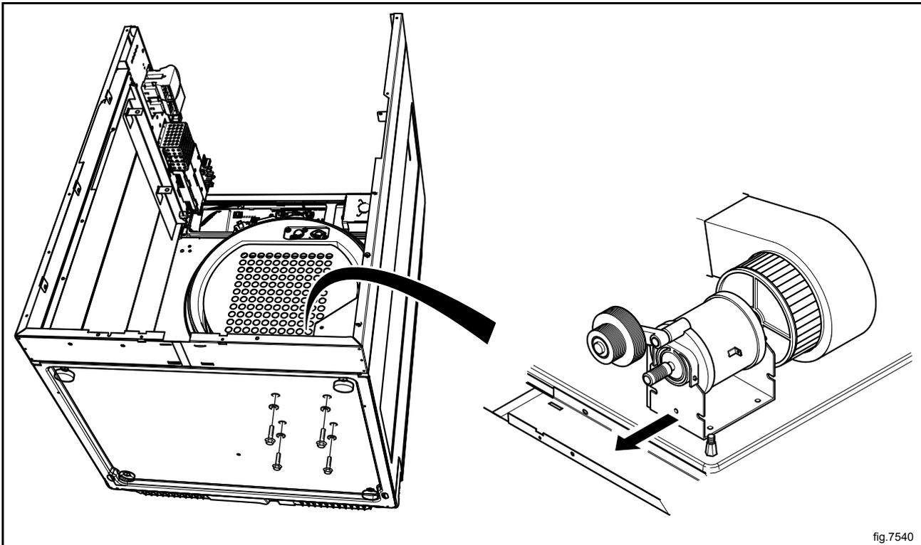
Demount the fan from the motor by loosening the set screw. The set screw can be accessed through a hole in one of the blades.
