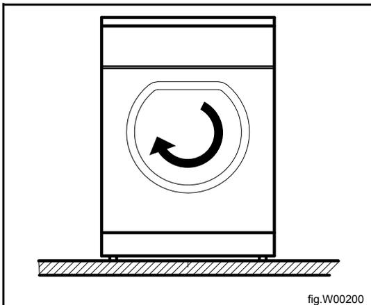
If the direction is wrong, swop two of the three phases to the left on the connection terminal.
