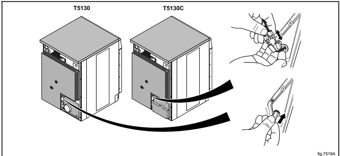
Demount the air channel panel. On condense machines: Pull out the hose to the drain from its upper connection.
