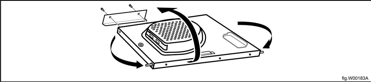
Demount the locking panels by loosening the barb with a screwdriver.
