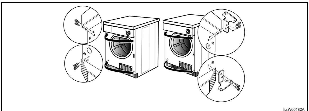
Demount the door handle and remount the screws. Mount the door handle on the opposite side using the existing screws.
