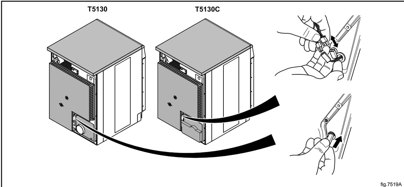
Demount the air channel panel. On condense machines: Pull out the hose to the drain from its upper connection.
