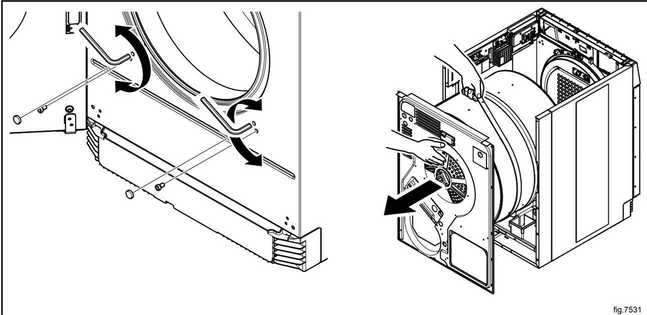
Remove the bolt and washer from the bearing to release the drum. Remove the rear panel from the old drum. Mount the rear panel with with the bearing on the new drum.
