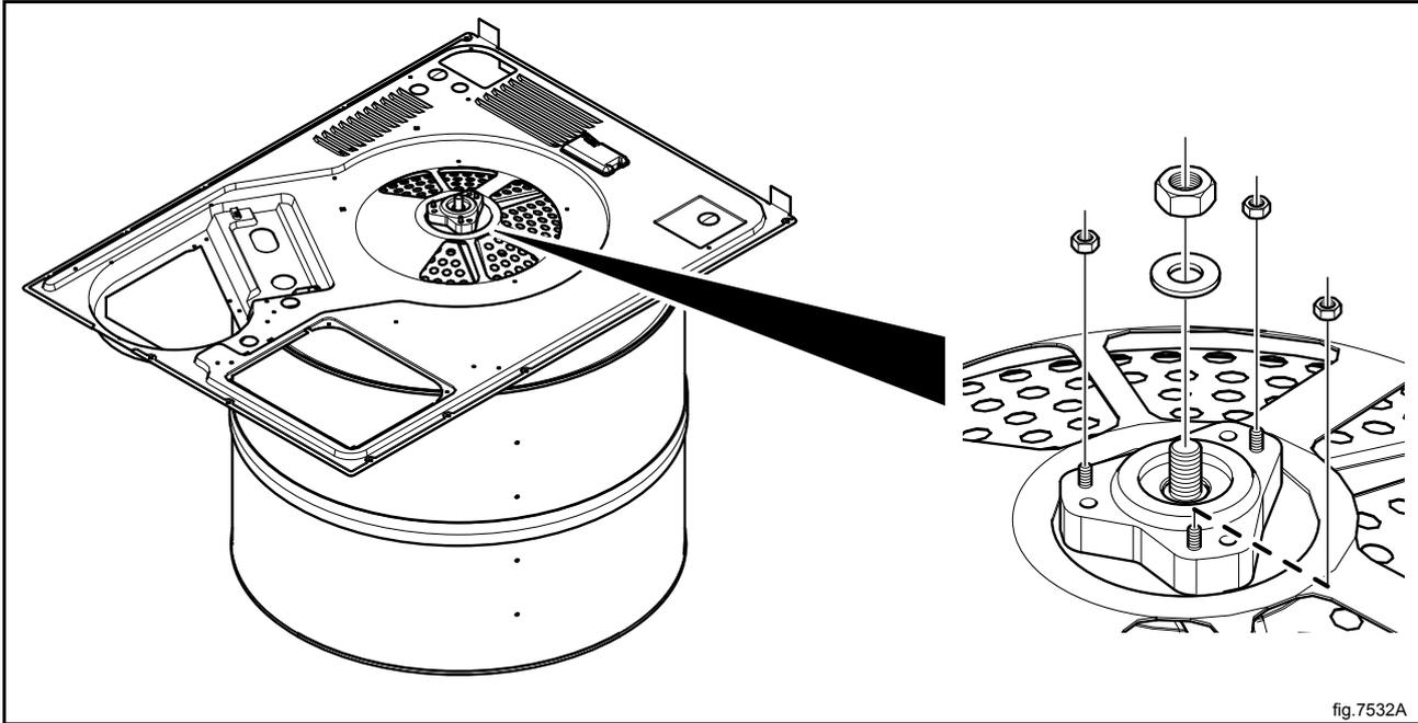
Carefully put the new drum package back in the machine.
