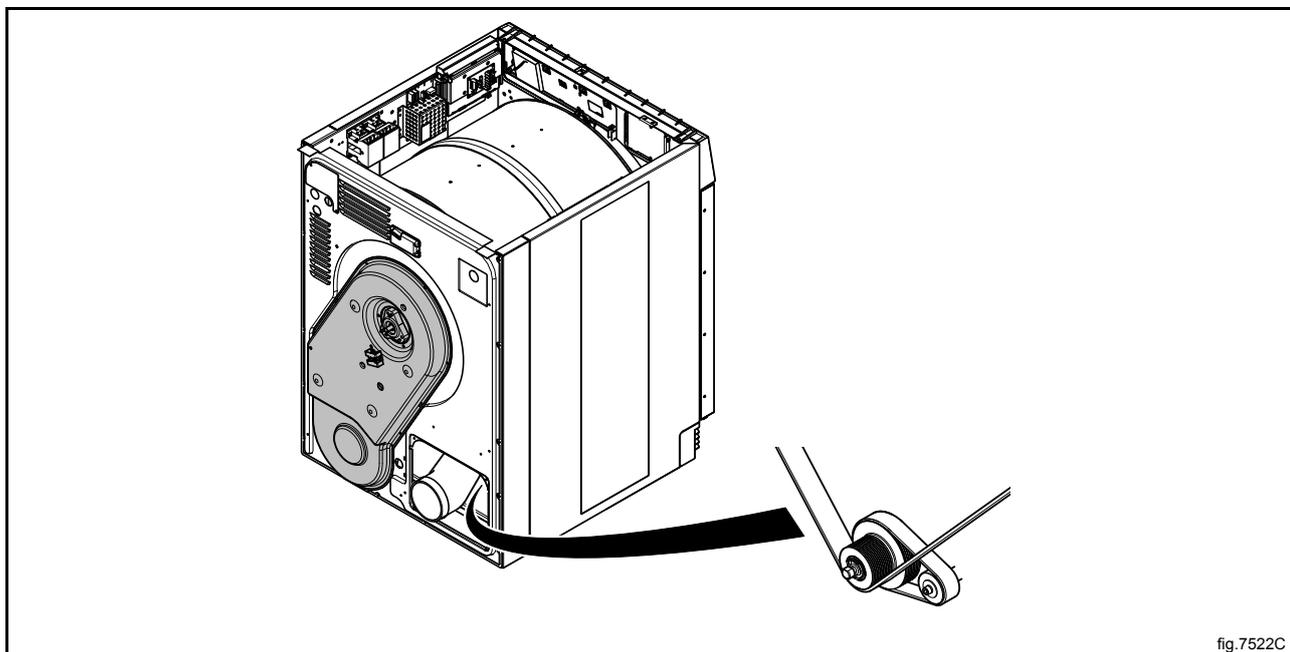
Unscrew the four screws at the panel around the heating element.
