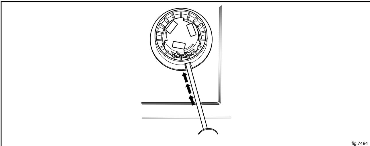
Mount the control knob on the inner knob. Continue to press with the screwdriver and turn the control knob clockwise until it stops when it is in position.
