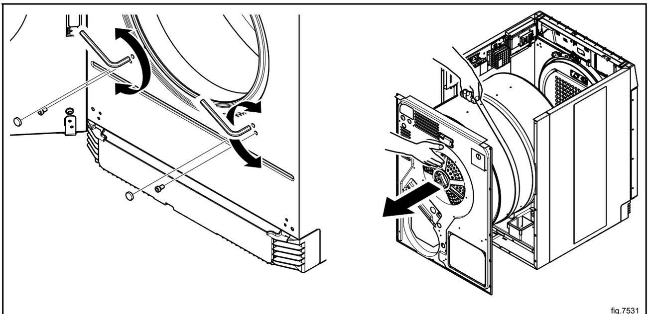
Remove the screws, bolt and washer on the bearing. Remove the bearing and mount the new one.
