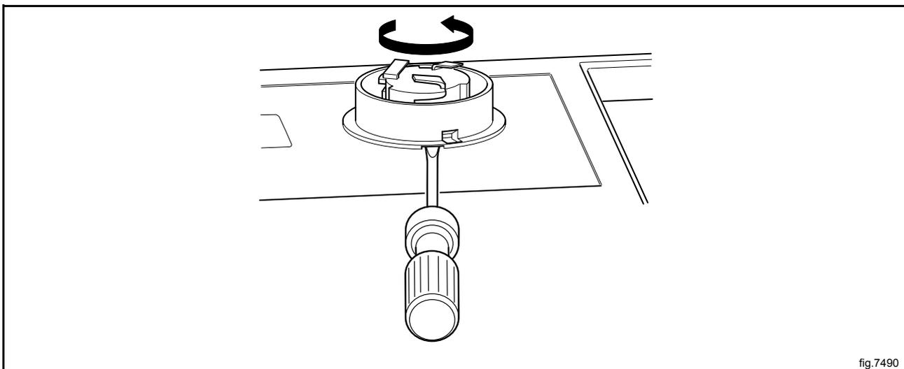
Mount the new cover ring and rotate it clockwise until it is in position.
