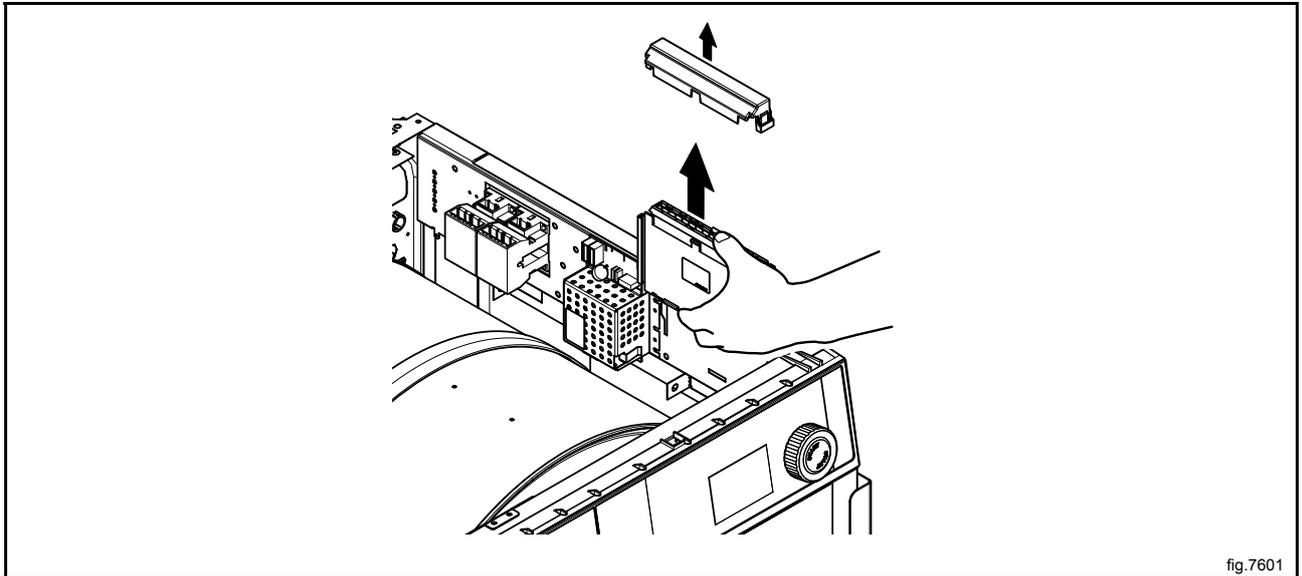
Insert the new module and make sure it is in position.
