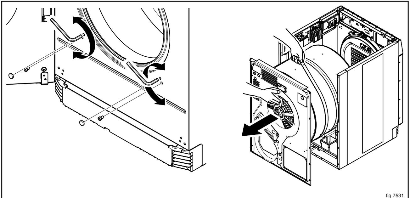
Carefully tilt the machine backwards and remove the three screws under the machine to release the lower element cover panel.
