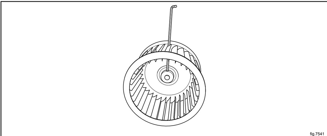
Mount the fan on the new motor and mount the new motor with the fan in the machine.
