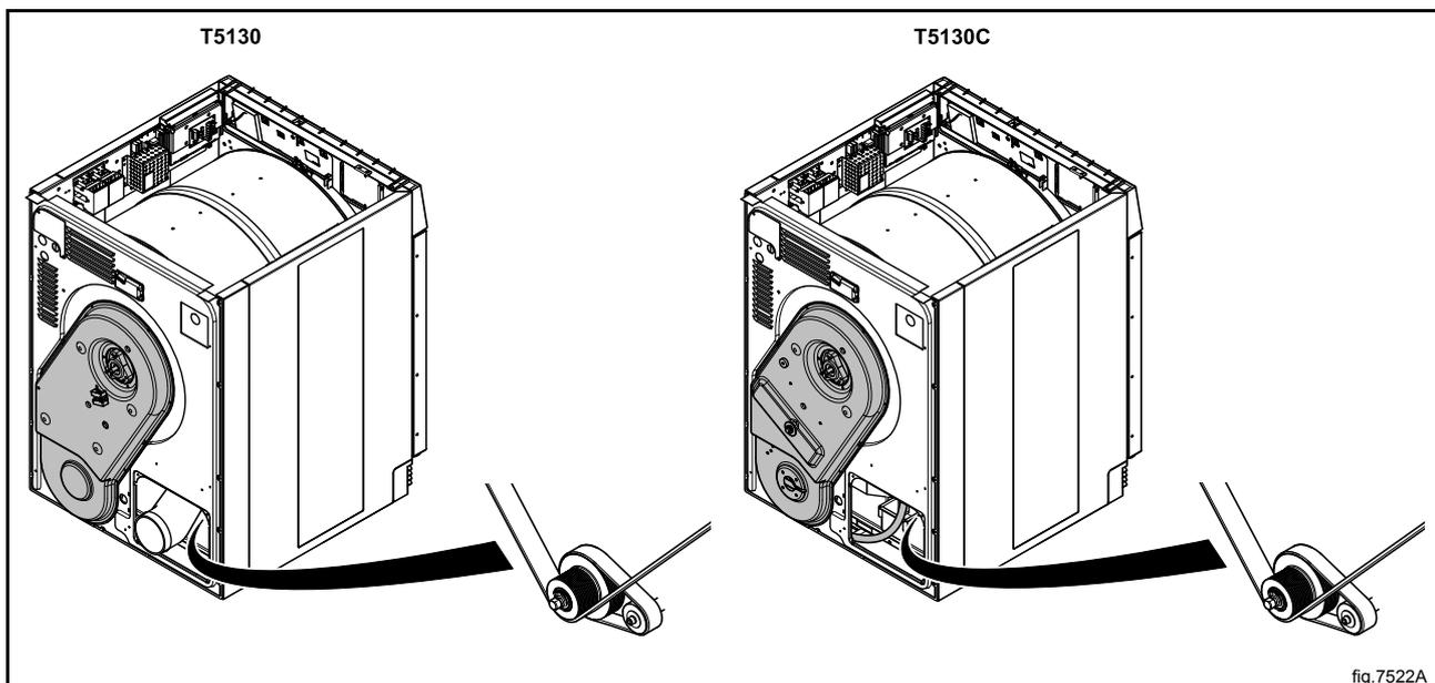
Unscrew the four screws at the panel around the heating element.
