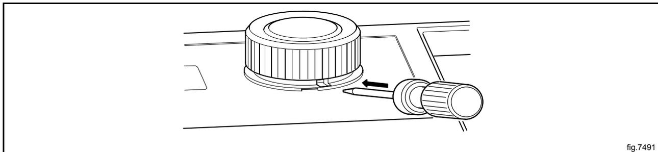
Gently push the screwdriver inwards and turn the control knob counter-clockwise until the screwdriver goes further in.
