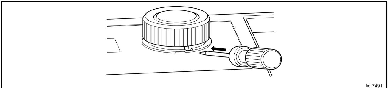
Gently push the screwdriver inwards and turn the control knob counter-clockwise until the screwdriver goes further in.
