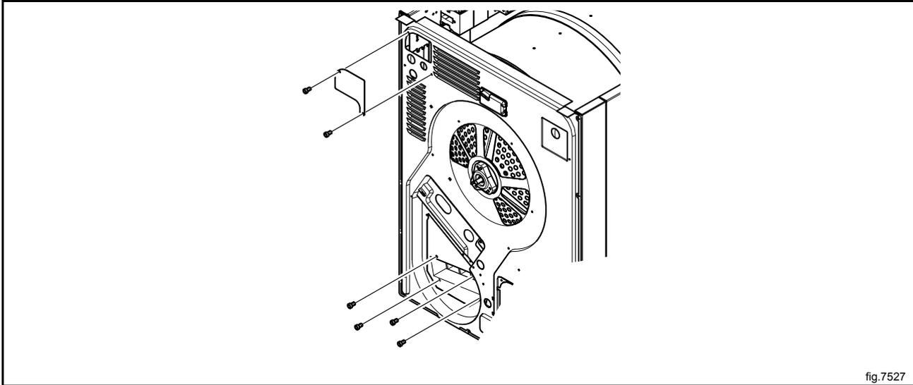
Unscrew the rest of the screws on the panel.
