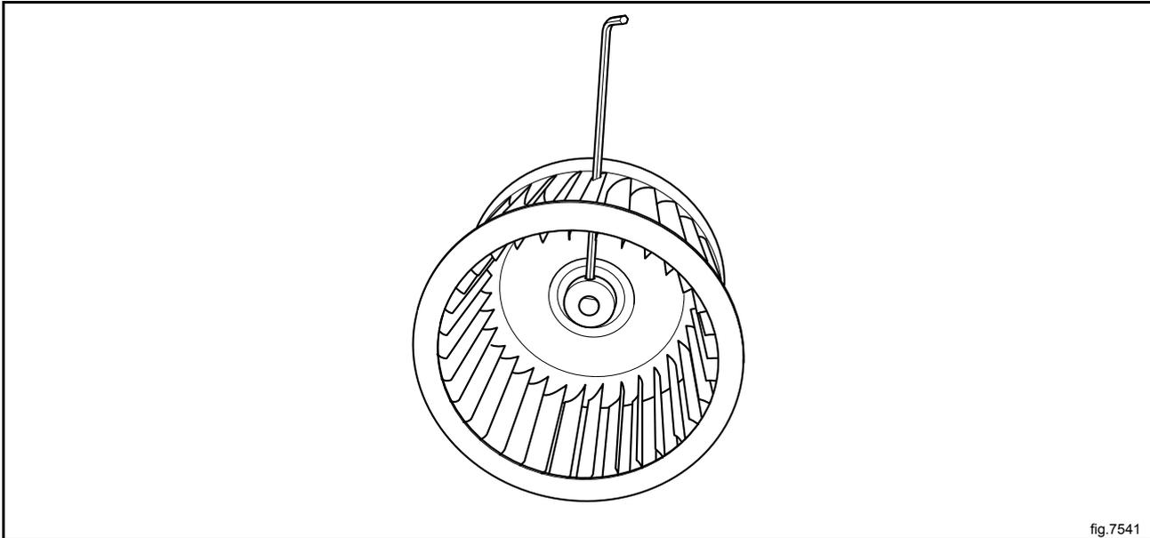
Use a puller to remove the fan from the motor.
