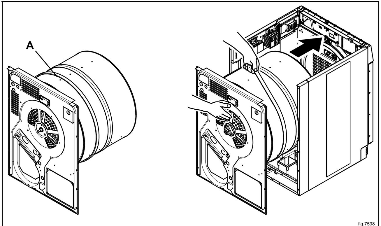
Fasten the support rollers at the front of the machine.
