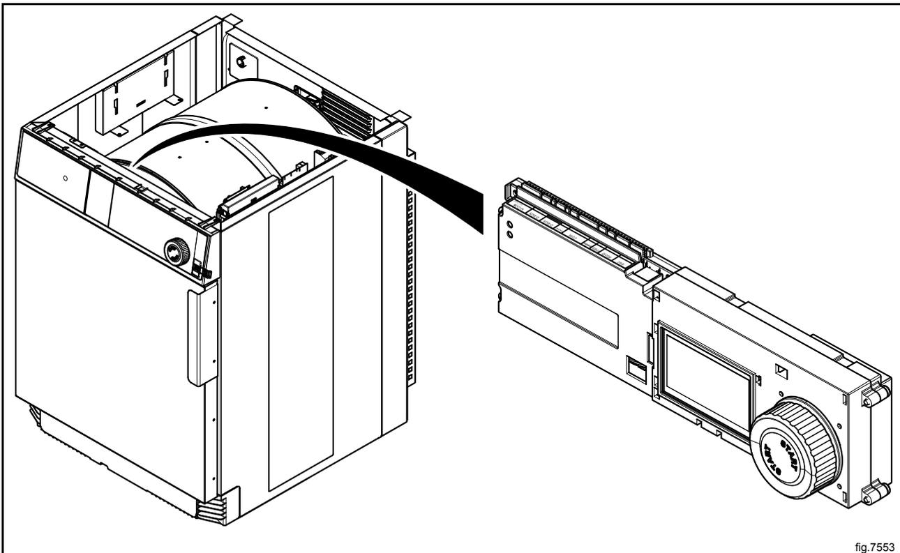
The program unit receives information from the I/O boards about input like temperature sensors, RMC, vacuum, door status etc, and output like drum, fan and heat control.
