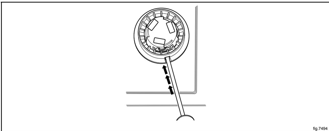
Mount the new control knob on the inner knob. Continue to press with the screwdriver and turn the control knob clockwise until it stops when it is in position.
