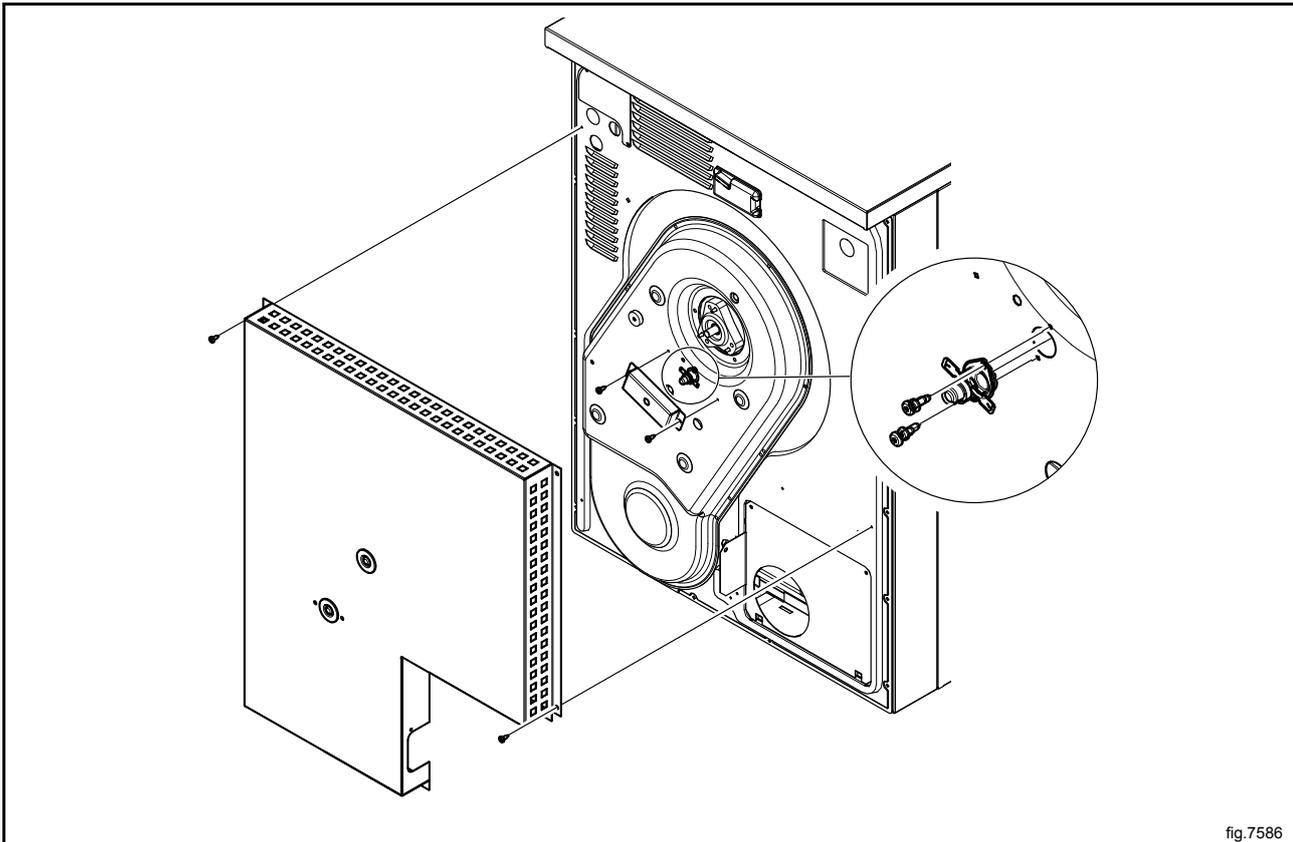
Remount the cover panel over the overheating thermostat and the rear panel.
