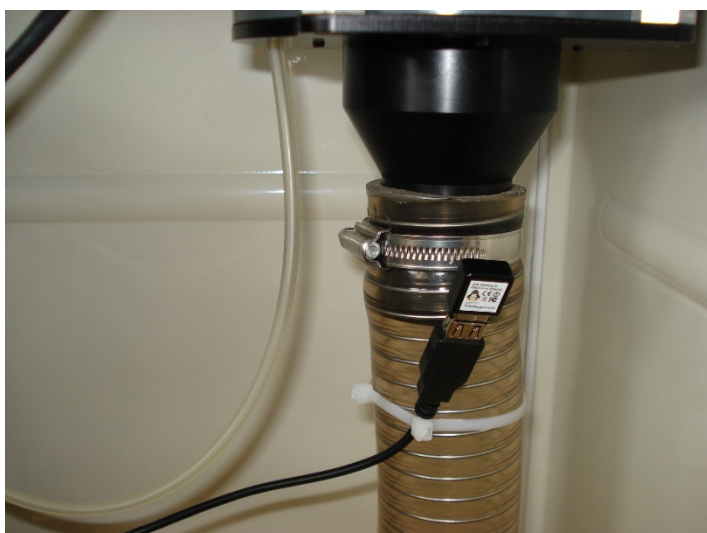
Install the end of the USB cable below the front test head (use a cable binder)
